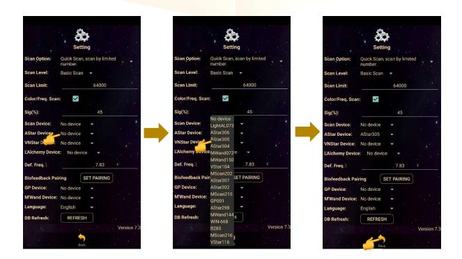
2. The icon of the device in the Home Page will turn on (turn to colour icon) when the device name is set in the application setting.
