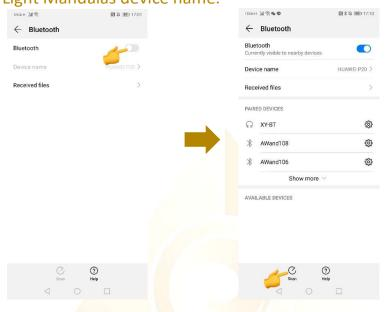
2. When the Light Mandalas device name appear, tap on it and insert password: "1234" then tap OK to pair it.
